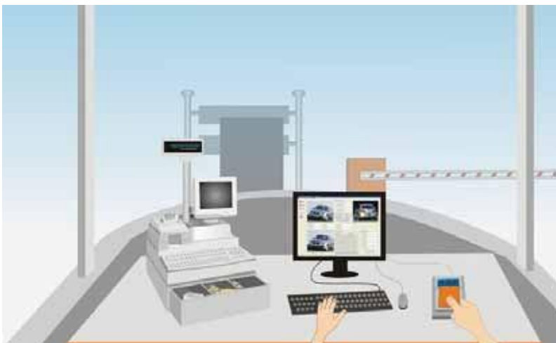
The security guard reads the RFID card with desktop reader, meanwhile the exit camera takes another picture of the plate Number
